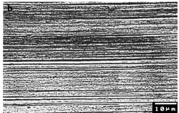
Figure 2 Microstructures of transverse (a) and longitudinal (b) sections of Cu-9 Fe-1.2 Ag microcomposite wires.
